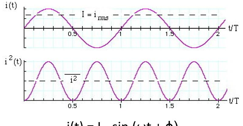
i(t) =  $I_m \sin(\omega t + \phi)$ where  $\omega = 2\pi f$
