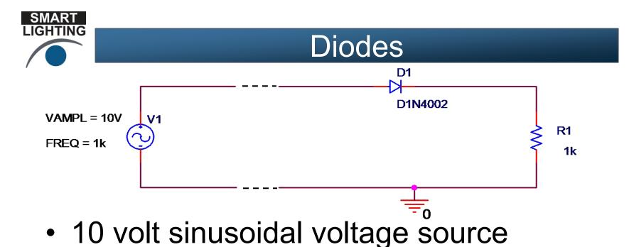
Connect to a resistive load through a diode
