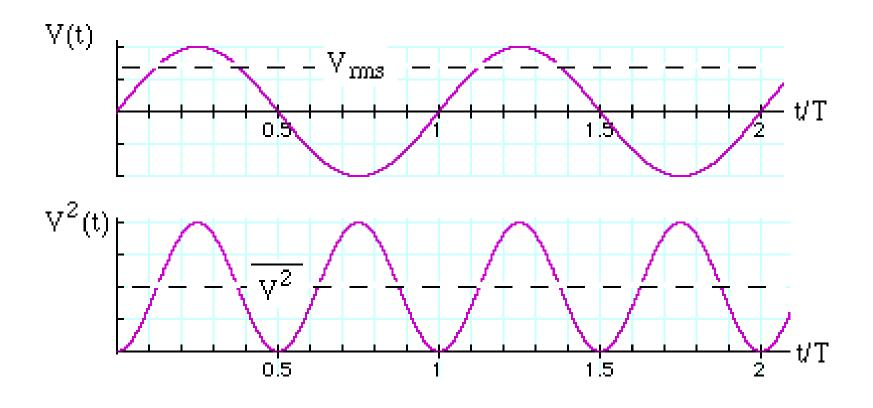
$v(t) = V_m \sin(\omega t + \phi)$ where  $\omega = 2\pi f$
